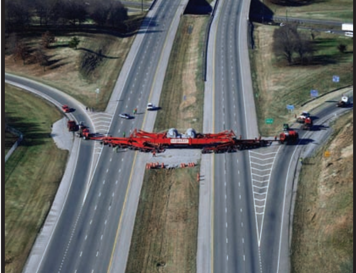
Barnhart Crane & Rigging Co. (No. 62) used a 345-ft-long transporter to haul a 660-ton generator from Forks in the River Industrial Park to a new powerplant near Rogersville, Tenn., for the Tennessee Valley Authority.
